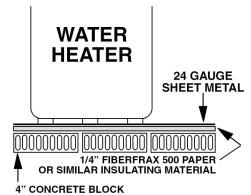
Minimum clearance to combustible construction is: SIDES 6"; BACK 6"; FRONT 24". The installation of this water heater must conform with local codes and ordinances. In the absence of local codes, the installation must comply with the National Fire Protection Association (NFPA 31) Code or CSA B139.
