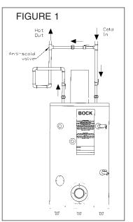
A thermostatically controlled anti-scald valve meeting requirements of CSA B125 or ASSE 1016 or 1017 should be used to temper the domestic hot water supply to fixtures to 49°C (120°F). See Figure 1 for proper installation of antiscald valve.
